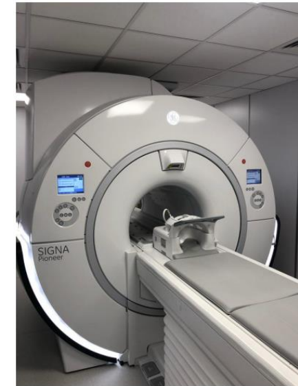
Figure 1: The equipment used in this study - 3.0 T Signa Pioneer MRI scanner produced by GE Healthcare
